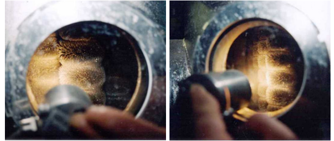
Typical particle build-up around the poles of the PACMAN magnetic elements
